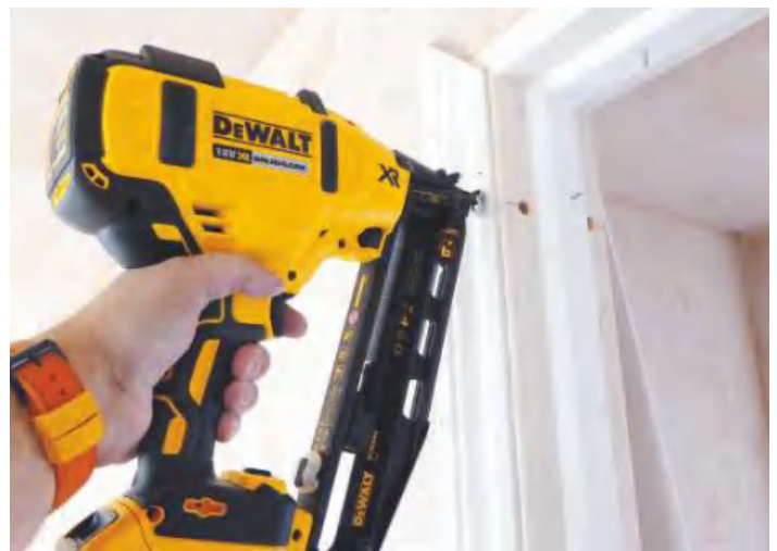
▲ Second fix work is where this gun excels, setting each fixing consistently
